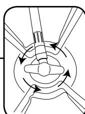
5. Open the valves completely by turning the valves COUNTER CLOCKWISE. Top flap may be removed or left in place during use or storage.
