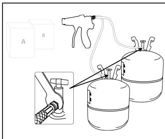
2. Thread red coded hose to A-component tank and black coded hose to B-component tank and tighten with supplied 9/16" wrench.
