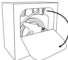
3. Push in top of front panel to open. Pull down flap for dispensing unit hose assembly. Remove nozzle packet and read instructions.
