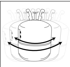
1. Shake each cylinder for 1–2 minutes before use to ensure proper mixing, see TDS for formula specific shaking and temperature recommendations. Chemical should be between 75–85°F (24–29°C).
