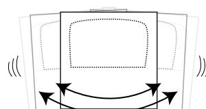
2. Shake kit for 1–2 minutes before use to ensure proper mixing. Typically chemical should be between 75–85°F (24–29°C). see TDS for formula specific shaking and temperature recommendations.
